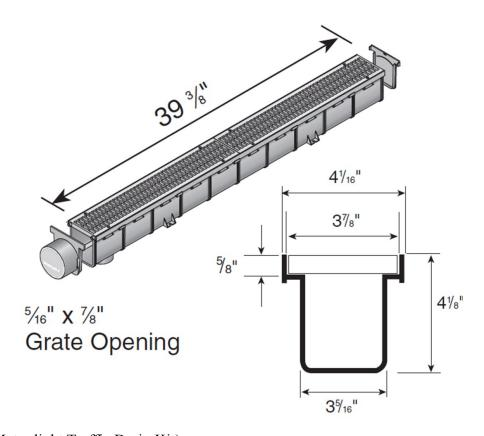
Part #: 764 ( 3" x 1 Meter light Traffic Drain Kit) Material: Channel PVC, Grate PVC, Cap/End Outlet
